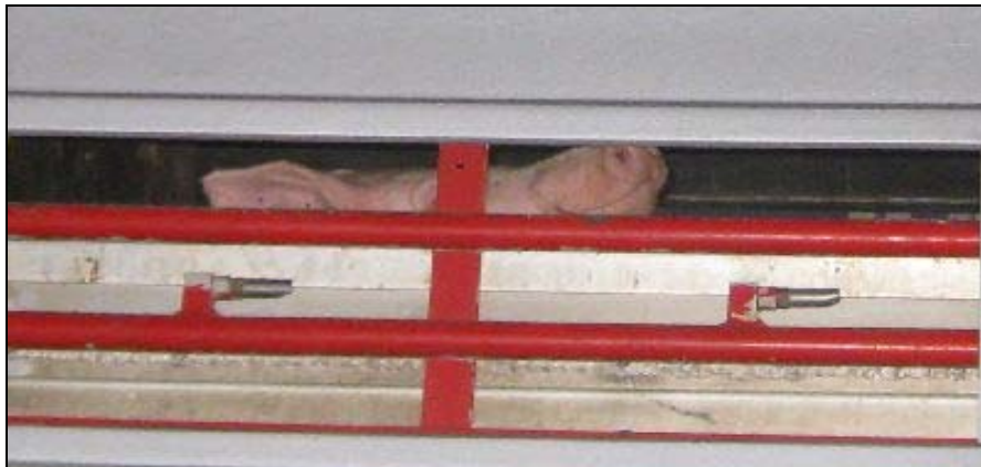
Second deck - Water nipples out of reach for the pigs – pigs remain without water for approx. 18 hours during summer.
