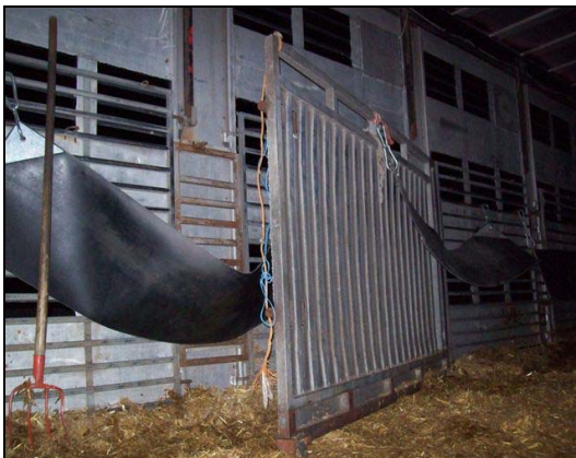
Metal dividers and inadequate rubber mats used as dividers in empty truck
